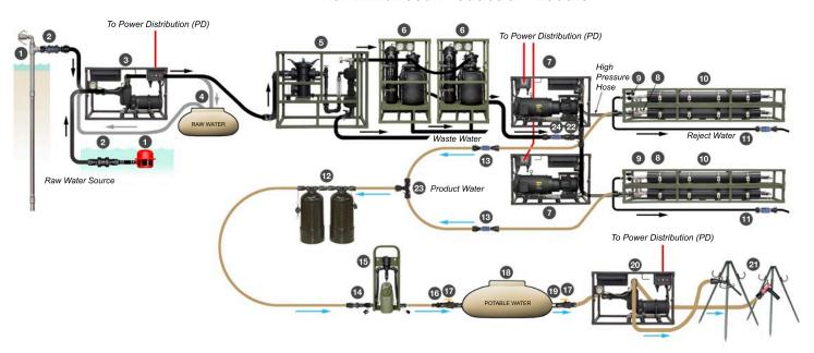
The E-LWPS EPM, (Lightweight Water Purification System - Enhanced Production Module), is the fifth extended capability module which can be added to the system to produce up to twice the water production with a significant fuel reduction.
