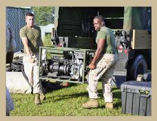
Lightweight - 2 person lift for every module. Pack out and operational in less than 40 minutes with only one operator required.
